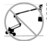
Do not place or attach fixed or overhanging loads to any part of this machine.
